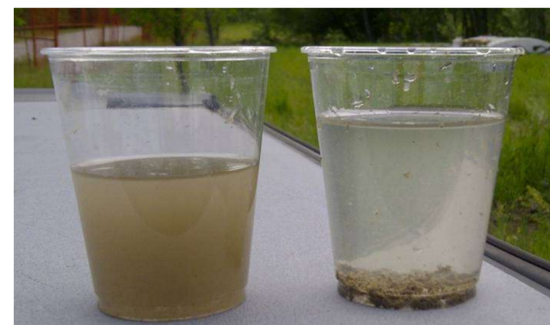
Left: Tailing pond water with TSS. Right: water sample treated with CC
